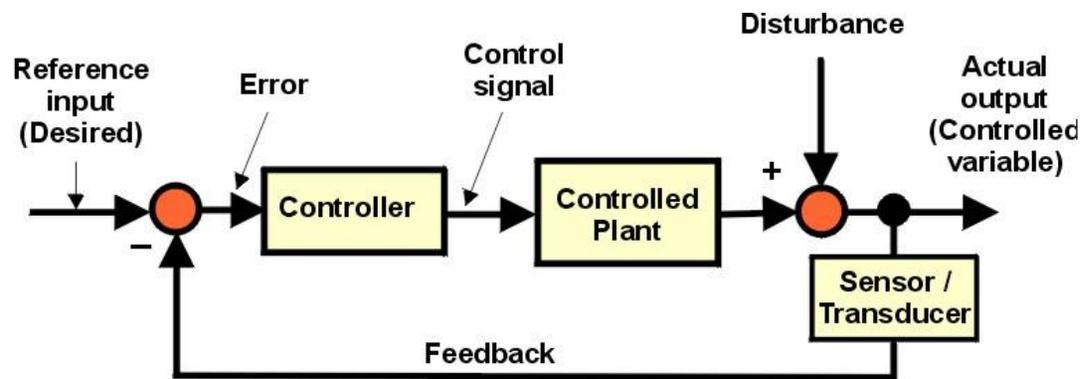
Fig.15: Feedback control system
